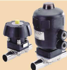
Type 2031 Pneumatic Operated Type 3233 Handwheel Operated Forged Stainless Steel, 2/2 way, Diaphragm Valve Orifice size : 8.0 to 100.0 mm Kv : 1.0 to 235.0 m³/h Port conn. : Weld ends to DIN, BS, ISO, SMS Tri-Clamp to DIN, ISO, SMS, ASME (Other connections on request)
