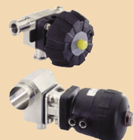
Type 2032 Pneumatic Operated Type 3234 Handwheel Operated Zero Deadleg T Diaphragm Valve Orifice size : 8.0 to 50.0 mm Kv : 1.0 to 51.5 m³/h Conn. Size : DN4 up to DN100 mm Port conn. : Weld ends to DIN, ISO, SMS, ASME, BS Tri-clamp to DIN, ISO, SMS, ASME (Other connections on request)
